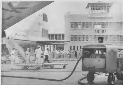
Link between hydrant and plane is the hose-cart in foreground. Visitors in background watch operations closely.
